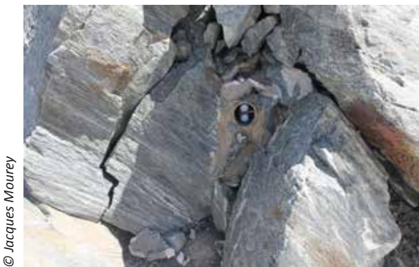
Figure 5. The pyroelectric sensor, camouflaged and sealed in a crevice on the edge of the “trail”.
